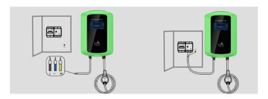
If a power distribution box is used, the L, N, and PE ends of the input cable of the plug correspond to the L, N, and PE ends of the circuit breaker respectively.
